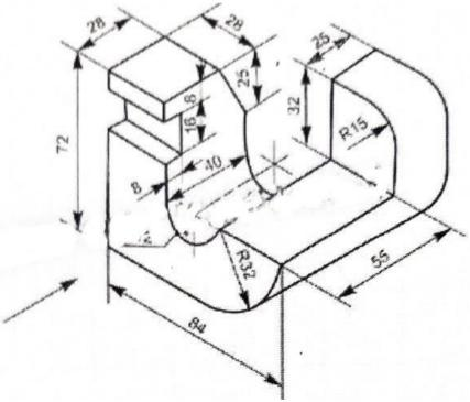
**4.** Figures show the isometric views of machine components and their view from the front, the view from above and the view from the right. Arrow indicates the direction to obtain the view from the front. Draw the orthographic views of the same. (10  $\times$  2)
