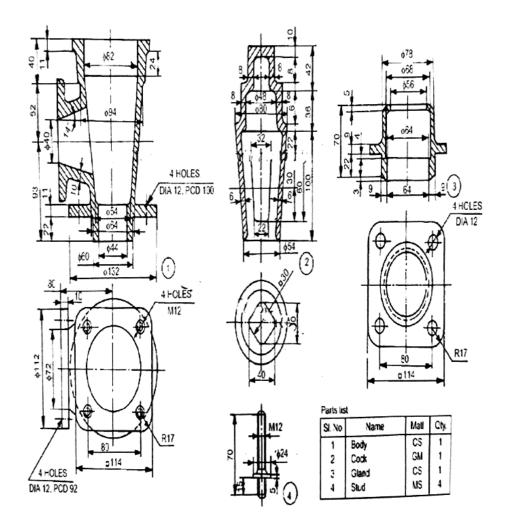
2. Assemble the parts of the feed check valve, shown in below and draw, (i) sectional view from the front, (ii) view from the right and (iii) view from above. (20)
